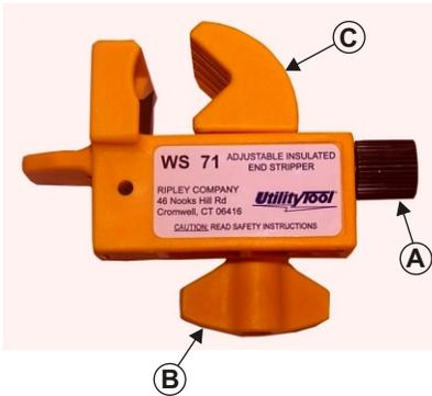
The Utility Tool WS 71 tool will end strip 600 volt insulated wire, including USE, THHN, XHHW, and other constructions. The tool's cable size range is .5" - 1.3" OD; 1/0 to 1000mcm conductor.
