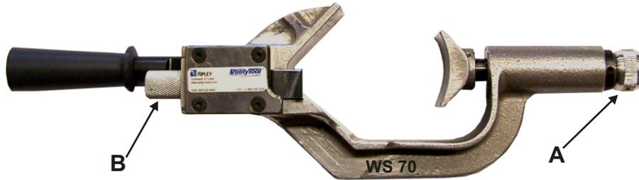
**NOTE:** The WS70 tool has been specifically designed for the removal of the polyethylene or PVC outer jackets on 46-69 KV high voltage transmission cables. The tool is also an adjustable end stripper for the same cable.
